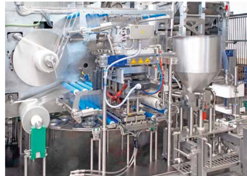
Photos at the top: Rotary-type cup filling machine GRUNWALD-ROTARY 12.000 with connected mobile fillers GRUNWALD-FLEXODOS and GRUNWALD-SEMIDOS (in the background) for filling non-pumpable salads
